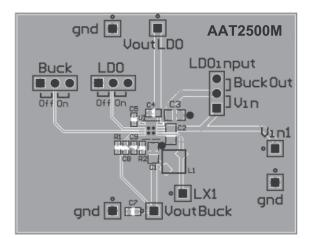
Figure 3: AAT2500M Evaluation Board Top Side Layout.
