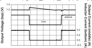
Step-Down Converter Load Transient Response (1mA to 400mA;  $V_{IN}$  = 5V;  $V_{OUT}$  = 1.2V;  $C_{OUT}$  = 4.7µF;  $C_{FF}$  = 100pF)
