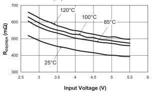
Step-Down Converter N-Channel R<sub>DS(ON)L</sub> vs. Input Voltage
