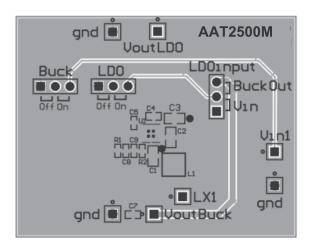
Figure 4: AAT2500M Evaluation Board Bottom Side Layout.
